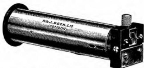
Figure 43. Prism spectroscope No. 2458 made by R. & J. Beck, London
